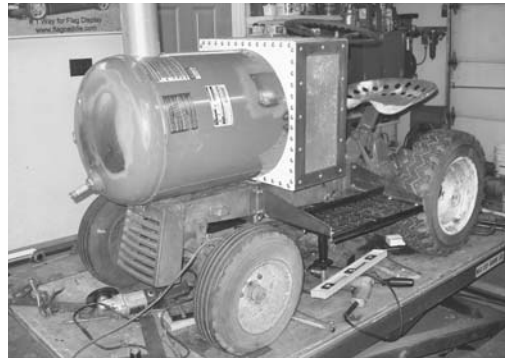
Doug Schiller built this mini antique steam tractor out of an old Sears garden tractor. He also built a 2-wheeled trailer to pull behind the tractor.
